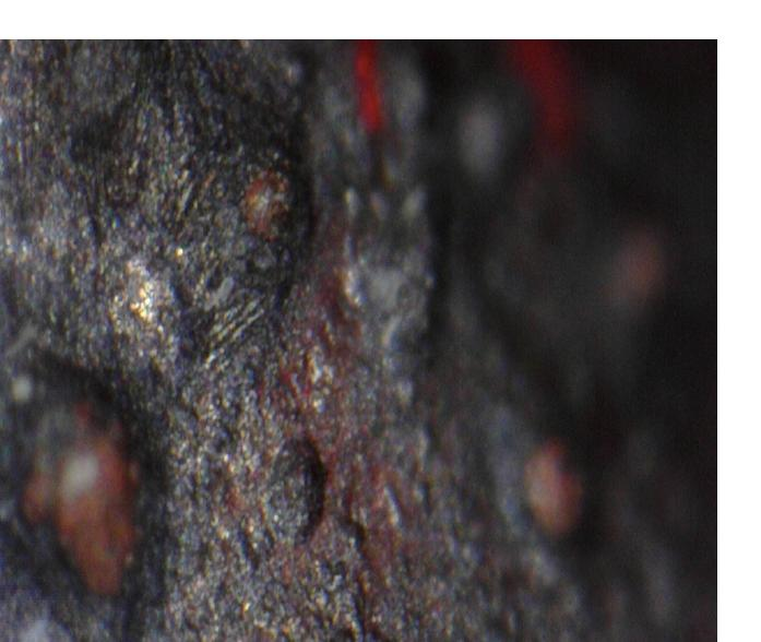
Microscope Picture of Cu sample after electrolysis
