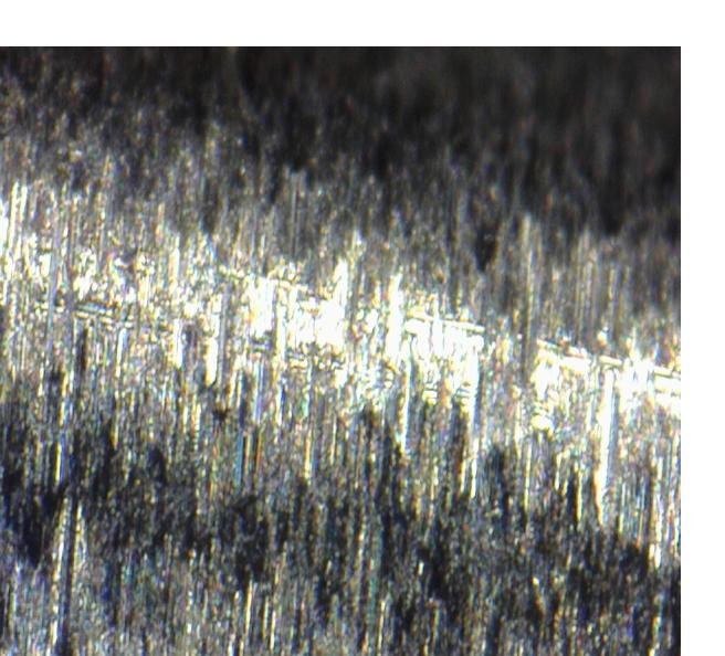
Microscope picture of Tungsten After pure Water electrolysis
