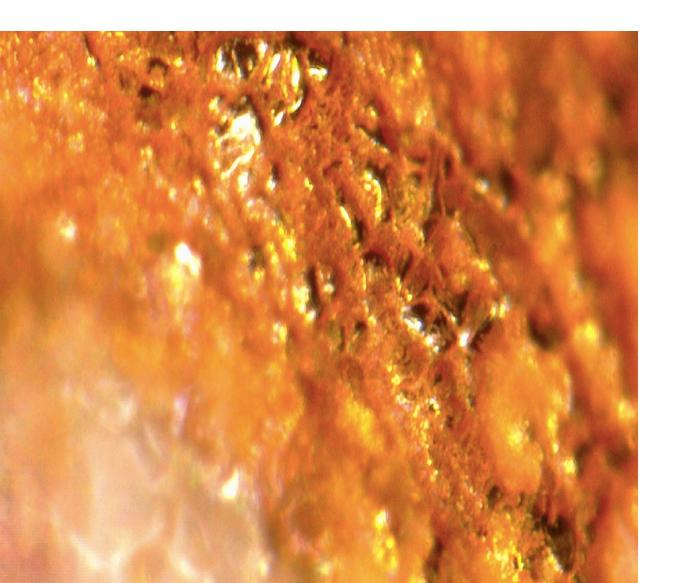
Microscope picture of the split off piece of Cu during electrolysis
